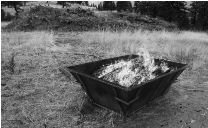
A custom kiln on private forest land in the Blackfoot Valley burns logging residues to create biochar, a highly absorbent porous substance similar to charcoal which can be used in remediation of water and soil contamination as well as improving soil fertility. The kiln was manufactured in 2017 by students in Missoula's Hellgate High School's welding class. Photo by: Martin Twer.
