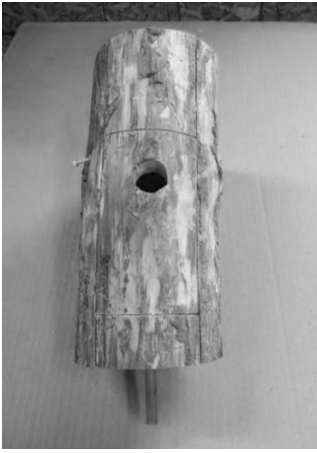
Figure 6: Peg in place on bottom. Notice nail inserted in pre-drilled hole left of the entrance.
