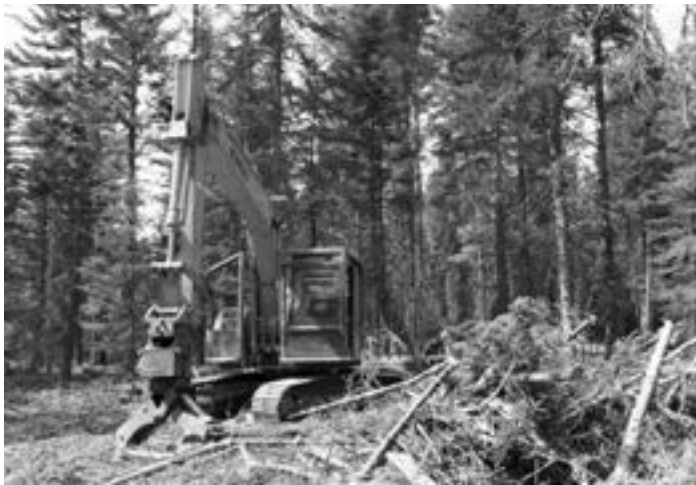
Log Loaders like this can be used to pile treatment residue for burning.
