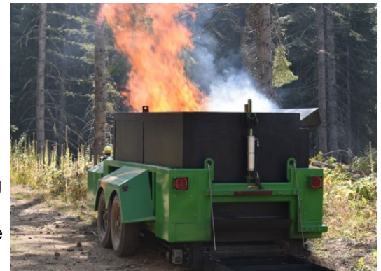
The CharBoss is an air curtain burner-style mobile biochar production machine that can consume material from most burn piles with minimal to no preparation. USDA photo by Darcy Weseman.
