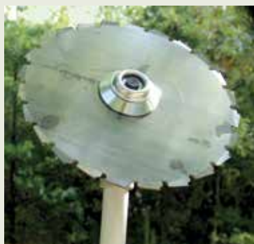
Brushsaw blade with chainsaw-like teeth.
