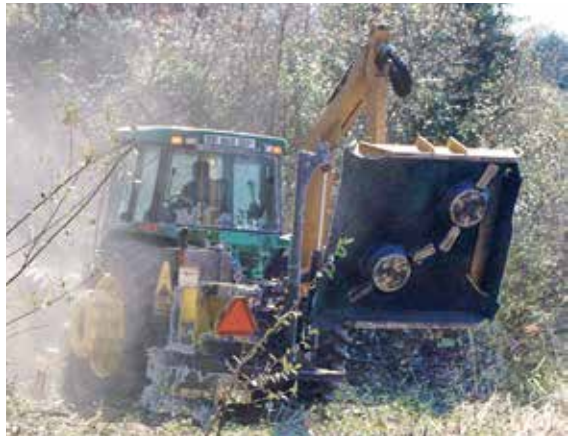
Wetblade system with two cutting heads.
