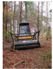
Mulching machine with horizontal shaft and rigid cutting teeth.
