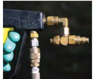
Spray gun with rollover valve that holds two tips.
