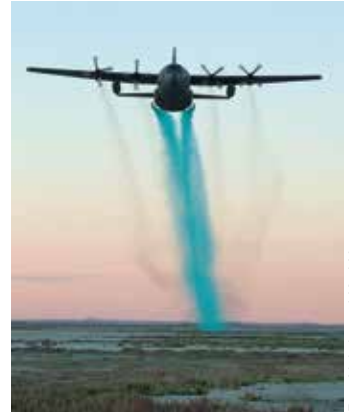
C-130H aircraft and Modular Aerial Spray Systems (MASS).
