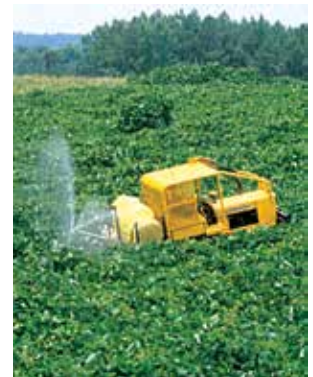
Boom Jet® nozzle on a crawler tractor spraying kudzu.
