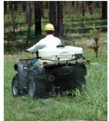
ATV mounted sprayer with a boom.
