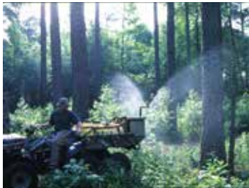
RTV mounted sprayer with Boom-Buster nozzles.
