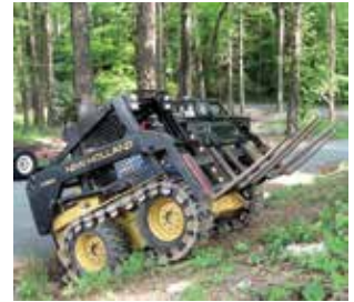
Skidloader with tracks and wider spaced pronged forks.
