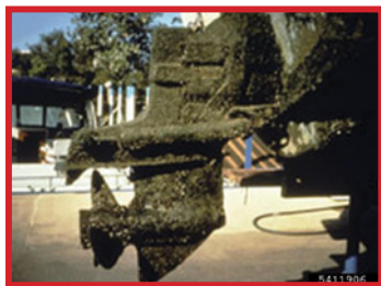
Zebra mussels can damage motors
