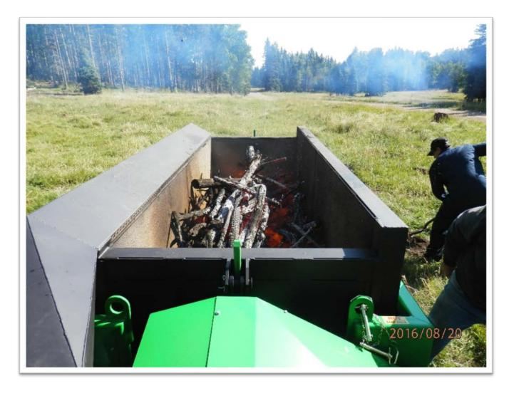
The photo (above) of the ACI shows the lack of smoke from the unit, but a large amount of smoke in the background from open burning on an adjacent lot. We are hopeful for a satisfactory resolution to the expense of the annual opacity test.
