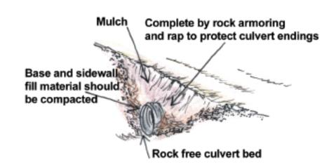
Install culverts at right angles to the stream. A maximum 15degree skew is allowed if approach conditions are difficult.
