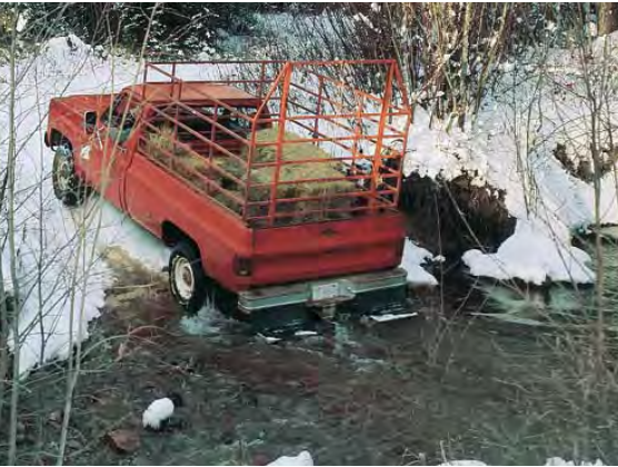
Fords are the least desirable stream crossing because of the continued disturbance to the streambed.
