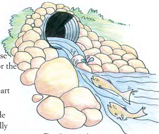
There's no pool below the inlet for fish to rest in or jump from.
