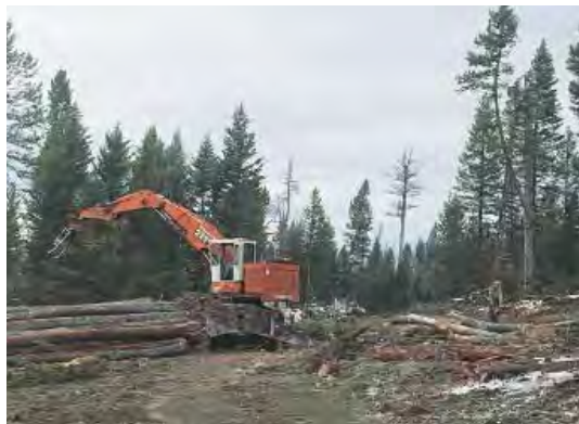
Roads dictate the location of log landings where logs are sorted and loaded on trucks. When roads use natural benches and flat areas, log landing excavation and sediment is reduced.
