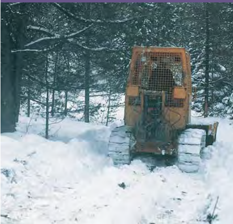
Compact skid trail snow before skidding logs. This avoids damage to soils that may be wet or not completely frozen.
