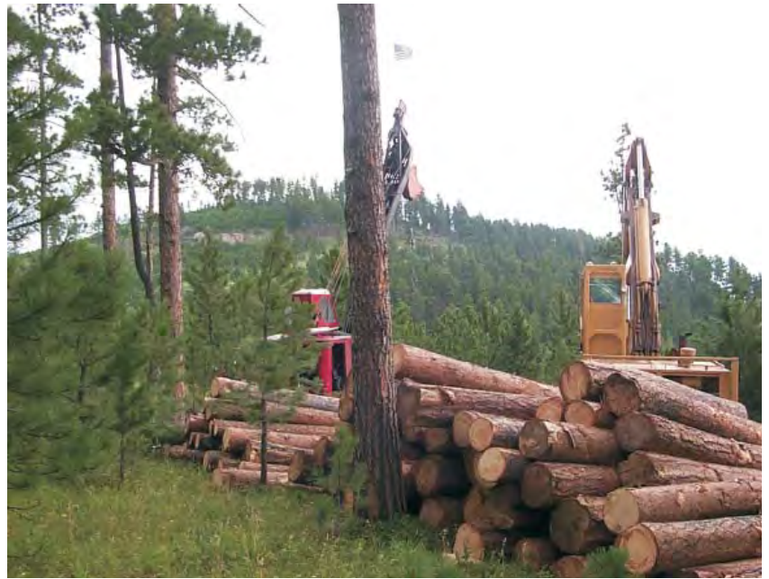
Trees are hand felled, limbed and bucked with chainsaws. A cable is stretched from the yarder to another point on the ground (stump, tractor, etc). The cable carries the logs over the terrain with either one end suspended or fully suspended, from where the tree is felled to the roadside or log landing. From there, logs are loaded on trucks. Yarders can reach out 1,000 to 2,500 feet.
