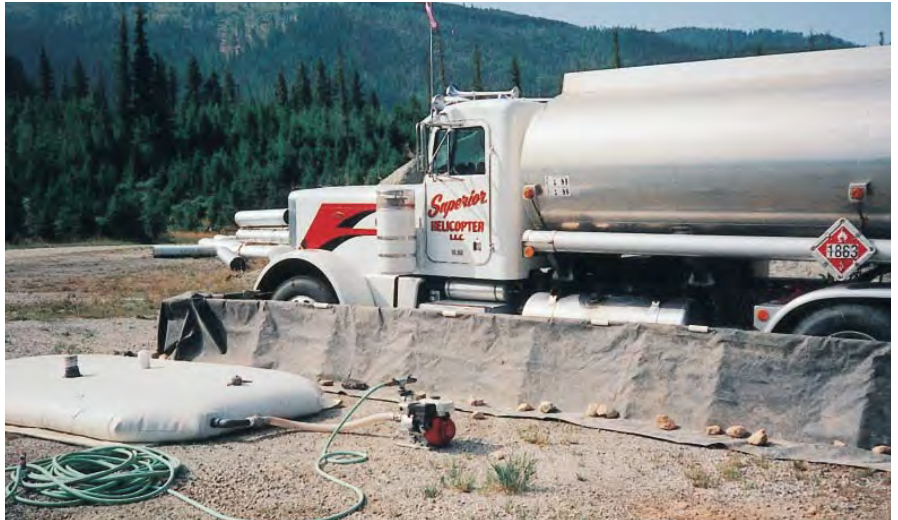
Helicopter service areas are located away from log landings. Operators are required to provide fuel truck containment in case of accidental spills. Portable water tanks and pumps are ready for fire emergencies.
