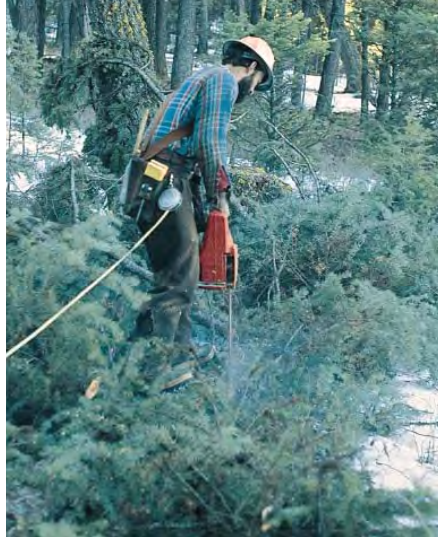
Tree felling, limbing and bucking are done with chainsaws.
